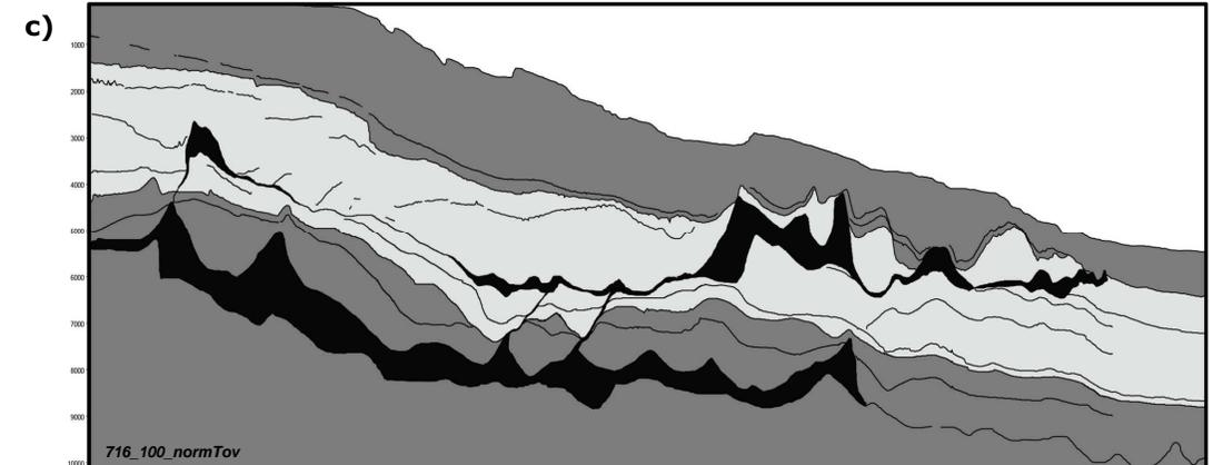
Figure 53: Three seismic lines across the study area: a) Line in the BSW area; b) line in the central part; c) line in the BaSW area. The Cretaceous series is shown in light grey.
