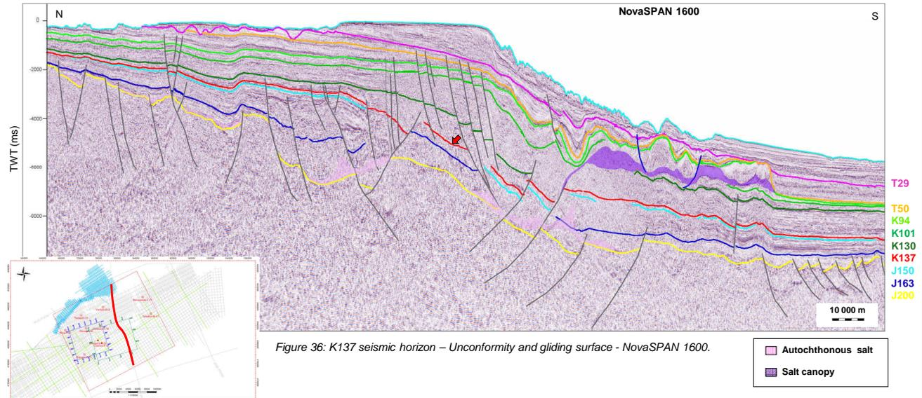
Figure 36: K137 seismic horizon – Unconformity and gliding surface - NovaSPAN 1600.
