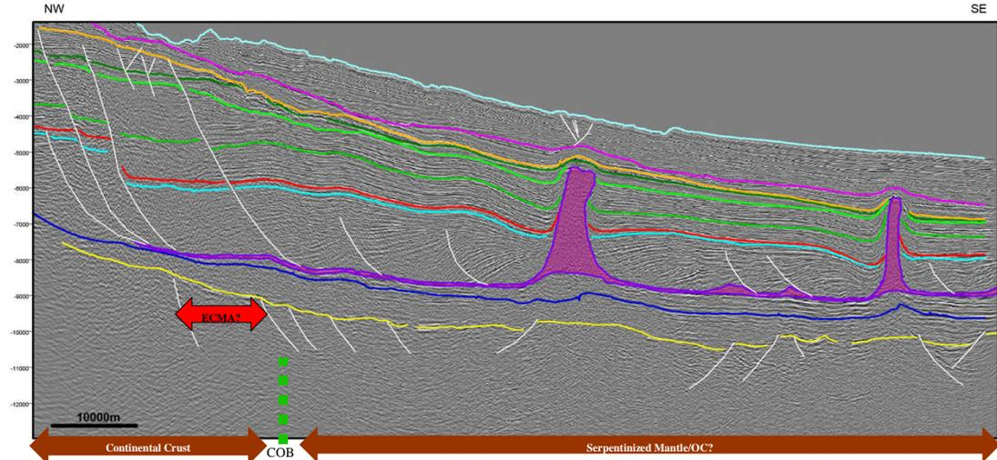
Figure 49: Base of Post-Rift Sediments – Banquereau Synkinematic Wedge area – 924-100 Norm Tov.
