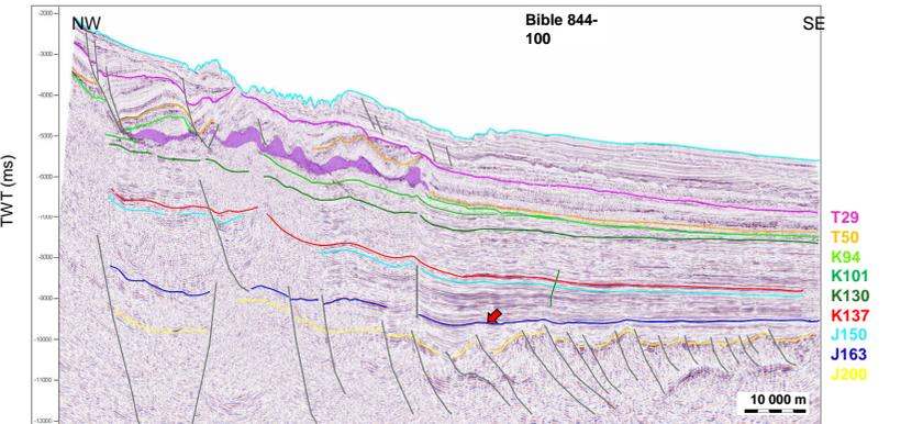
Figure 40: J163 seismic horizon - Bible line 844-100.
