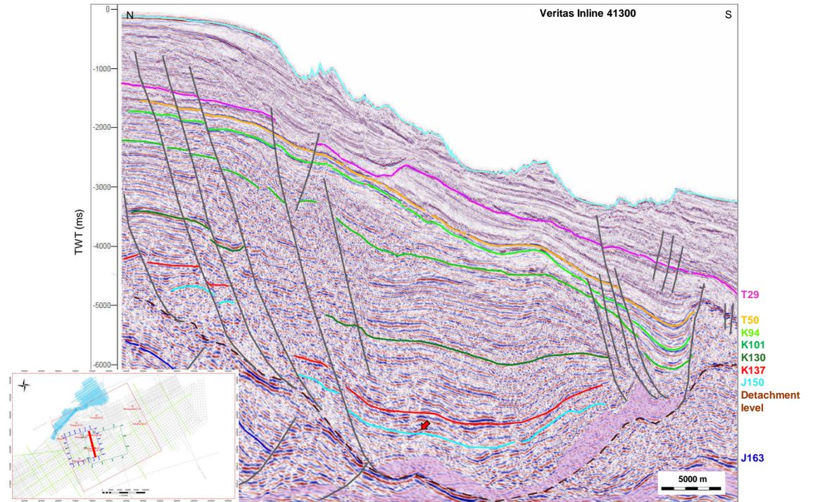
Figure 38: J150 seismic horizon – “Fishbone” structure - Inline 41300 in the Veritas 3D cube.
