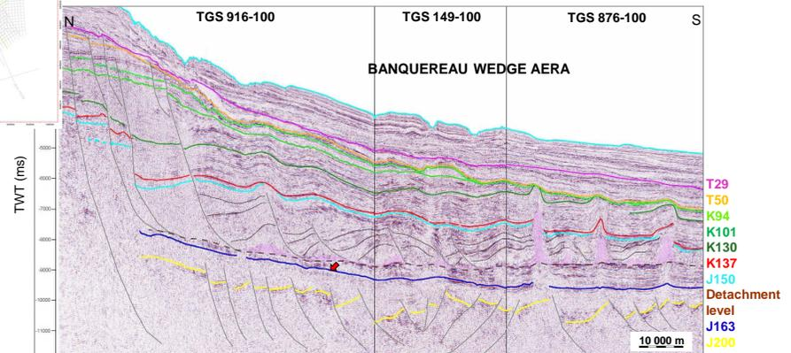
Figure 42: J163 seismic horizon - BSW area, composite line.
