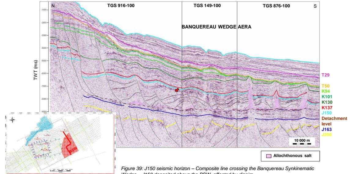
Figure 39: J150 seismic horizon – Composite line crossing the Banquereau Synkinematic Wedge – J150 deposited above the BSW, affected by diapirs.
