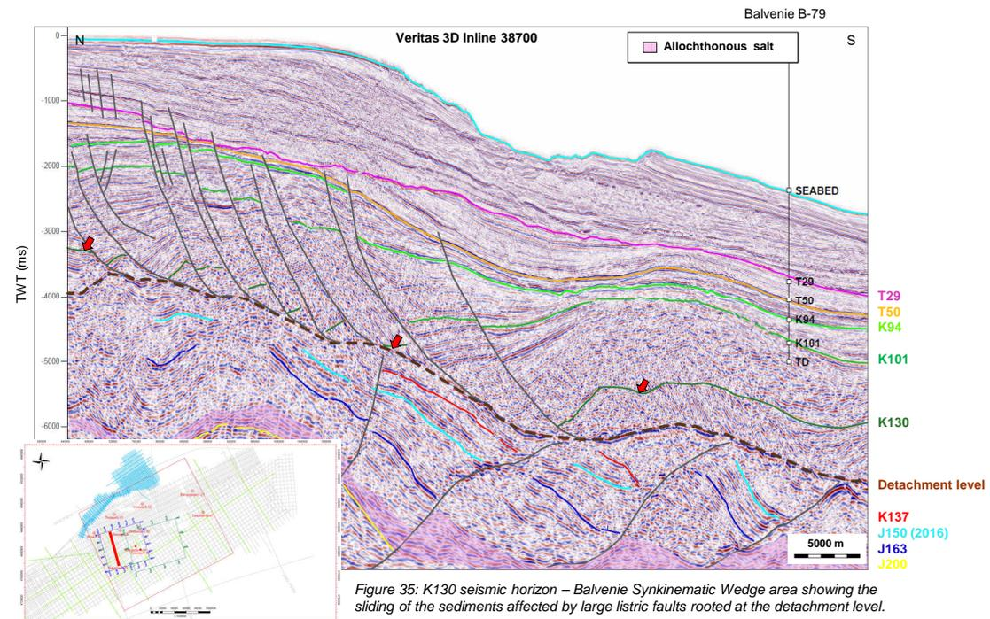
Figure 35: K130 seismic horizon – Balvenie Synkinematic Wedge area showing the sliding of the sediments affected by large listric faults rooted at the detachment level.
