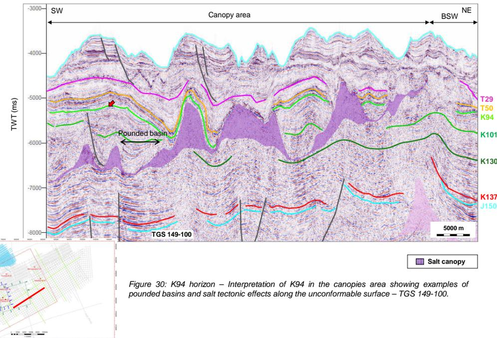
Figure 30: K94 horizon – Interpretation of K94 in the canopies area showing examples of pounded basins and salt tectonic effects along the unconformable surface – TGS 149-100.
