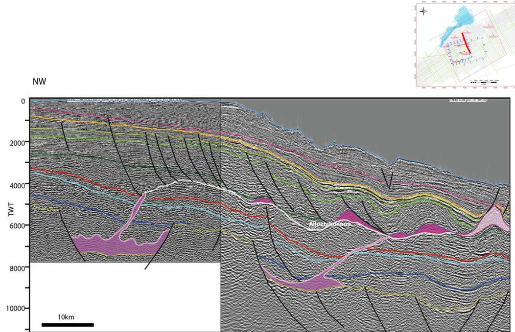
Figure 43: Allochthonous salt – Banquereau detachment wedge zone – composite 2D line (83-1030B mgr & 812-100 NormTov).
