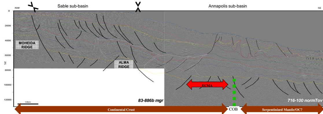
Figure 50: Base of Post-Rift Sediments\_ transition between continental and oceanic crust.
