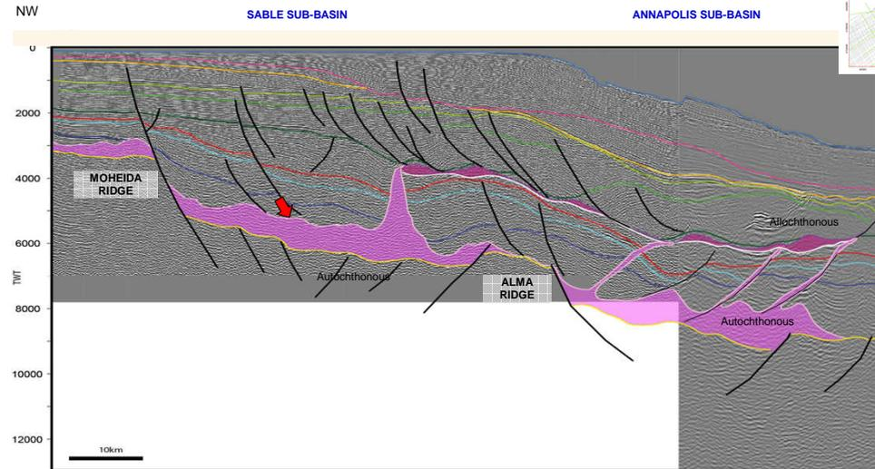
Figure 47: Allochthonous Salt - Sable Sub-basin – 2010 reprocessed GXT NovaSPAN 2D line 1600 – PSTM.
