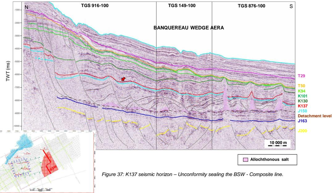
Figure 37: K137 seismic horizon – Unconformity sealing the BSW - Composite line.
