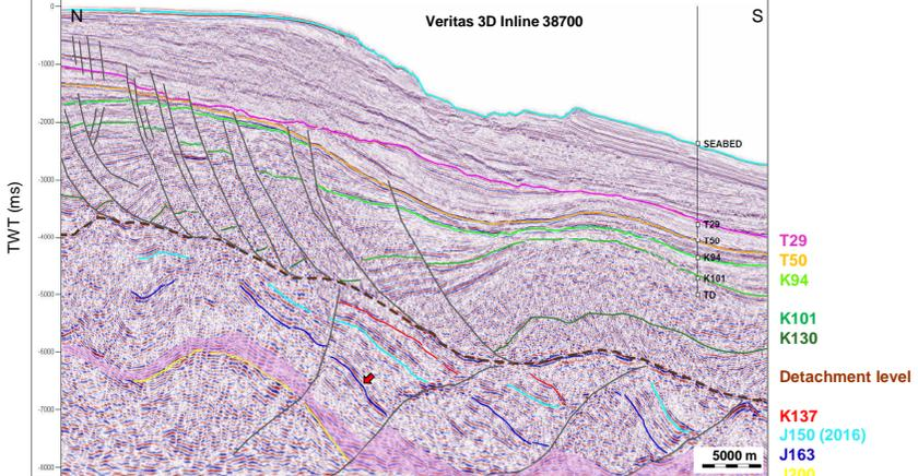
Figure 41: J163 seismic horizon - Line in Veritas 3D cube - Geometry of tilted blocks affecting the J163 horizon.
