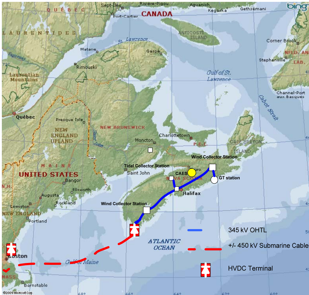
Figure 5-6 NS-NE HVDC Submarine Cable Consideration
