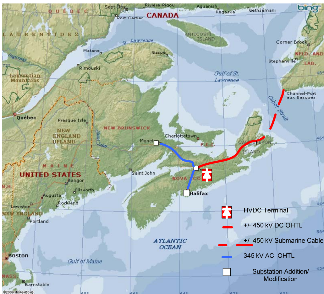
Figure 5-4 Illustrations of Transmission Requirements for Lower Churchill Imports
