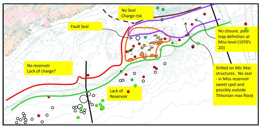
Figure 44: Main well failure modes
