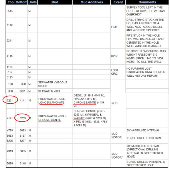
Figure 1: Glenelg J-48 - Example of a mud scheme used in many drilling operations
