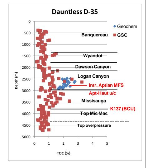
Like South Griffin J-13, Dauntless D-35 was drilled using Lignosulfonate added to the mud
