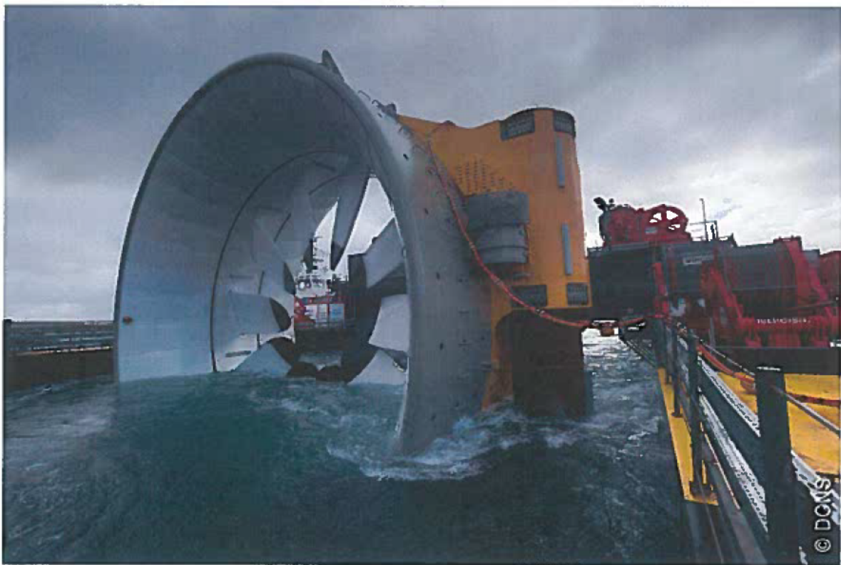
Figure 1: Open Centre Turbine on the deployment barge.
