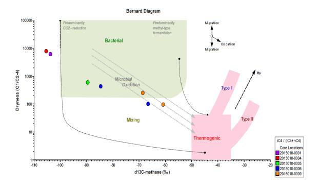
**Figure 1.** Plot of Methane Carbon isotopic value versus gas dryness displaying the possible mixing of thermogenic and biogenic methane in samples from sites 6 and 9. Note in order to be able to plot the pure biogenic gas samples from sites 1 and 4 on this figure, they were given a very low ethane concentration of 1 mole%.
