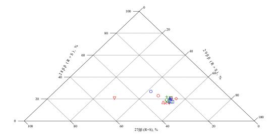
**Figure 2.** Relative abundance of  $C_{27}$ - $C_{29}$   $\alpha\beta\beta$  steranes in samples analyzed by GC-MS. Note the 2015018-0018 sample is drilling grease.
