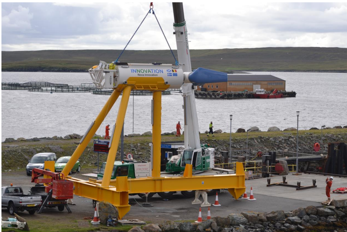
Figure 1 The Nova M100 Tidal Turbine sitting dockside before deployment in Shetland, UK
